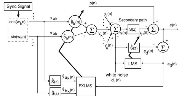
**Fig. 1** Block diagram of a conventional narrowband ANC system with secondary path modeling (the  $i$ -th channel).
