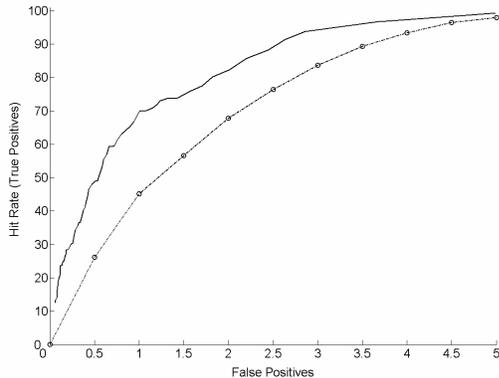
Fig. 4. Truncated ROC curves for the latest LF-ASD (Dashed line with circles) and our proposed design for subject 2 (Solid line).
