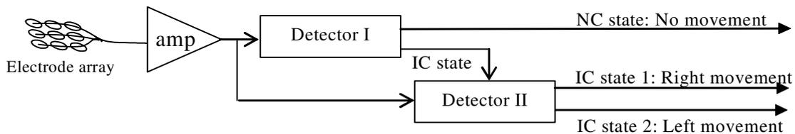
Fig. 1. Structure of the new 3-state asynchronous BI design
