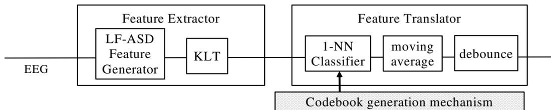
Fig. 2. Structure of Detector I, where KLT = Karhunen-Loève Transform, and 1-NN = 1-Nearest Neighbour.
