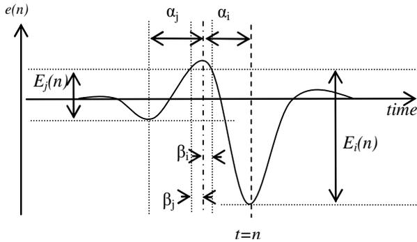
Fig 3. Description of delay terms ( $\alpha_i, \alpha_j, \beta_i, \beta_j$ )
