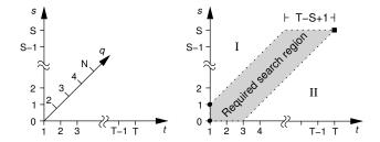
**Fig. 1.** 3D trellis (left) with time t, alignment s, and state q. 2D projection of this trellis (right), where the state axis is omitted. The 2D trellis shows the region that has to be calculated. Only points in this area can actually lead to a valid path through the model.
