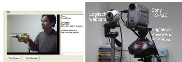
**Fig 1 (left)** is the illustration of multimedia synchronization based on object detection. **Fig. 2 (right)** is the camera system hardware
