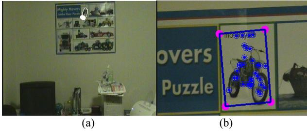
**Fig. 9** Distant-object recognition (a) detected laser pointer virtual ellipse, the white dot is the last detected point. (b) PTZ camera view after zoom-in, showing calculated object pose and matched SIFT keypoint
