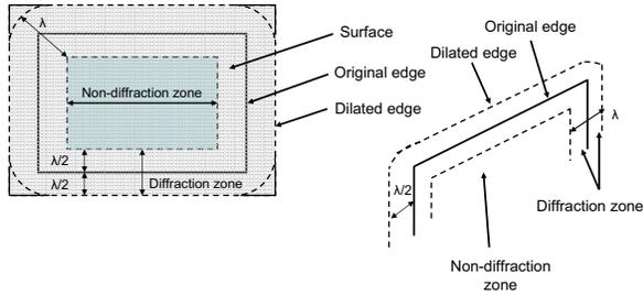
**Fig. 1.** Defining the diffraction and non-diffraction zones.
