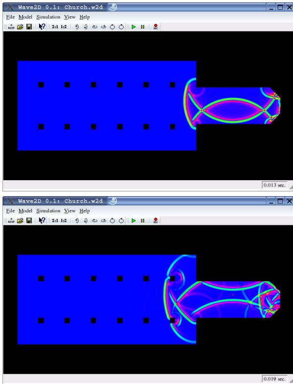
**Fig. 4.** Impulse propagation in a church simulated with “Wave2D”. Complete videos can be found in [6].
