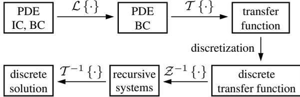
**Fig. 2.** General procedure of the FTM for solving initial boundary value problems in form of PDEs with initial- (IC) and boundary (BC) conditions. The transformations are explained in the remainder of this section.
