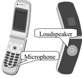
**Fig. 4.** Locations of Microphone and Loudspeaker on Hands-Free Cellphone.
