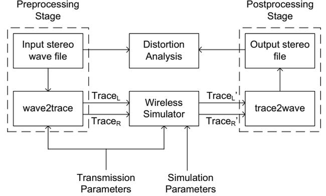
**Fig. 2.** Block diagram of the proposed wireless audio playback simulation methodology
