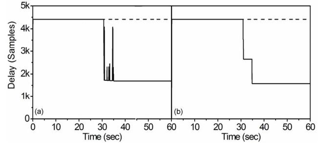
Fig. 4. Total playout delay for 11Mbps PHY under heavy interference, Simple Scheduler (a)  $L_f=294$ , (b)  $L_f=882$ . Dotted Line shows error-free transmission delay.
