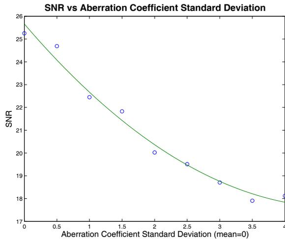
Fig. 7. SNR against aberration coefficient
