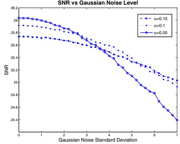
**Fig. 5.** SNR of the reconstructed image against level of noise corrupting the sub-images.
