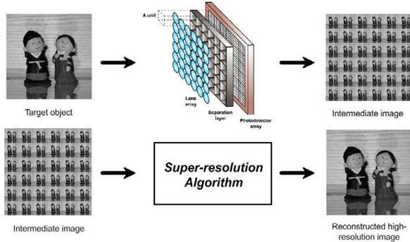
Fig. 2. Diagram showing the workings of the computational compound-eye imaging system.
