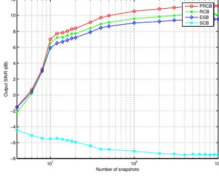
**Fig. 2:** Performance comparison of the beamformers with 3 impinging sources
