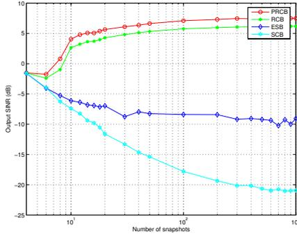
**Fig. 3:** Performance comparison of the beamformers with 7 impinging sources
