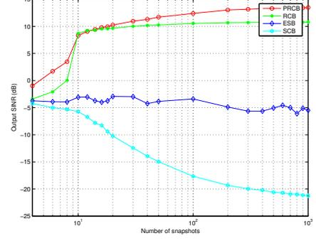
**Fig. 4:** Comparison of the output SINR of the beamformers versus number of snapshots with 3 impinging sources (The dimension of signal-plus-interference subspace is overestimated as 4. )
