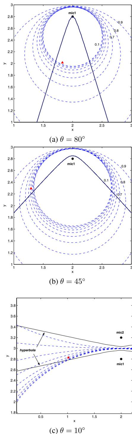
**Fig. 2.** Simulation results for proposed location method. The source is placed at three different directions with respect to array normal direction, and depart from array center one meter away. The reflection coefficient varies from 0.1 to 0.9
