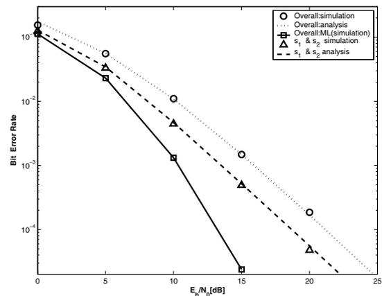
Fig. 3. Overall BER performance of the ZF-DF detector and the ML detector.
