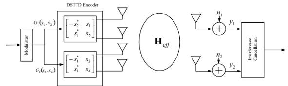
Fig. 1. Block diagram of a DSTTD system.
