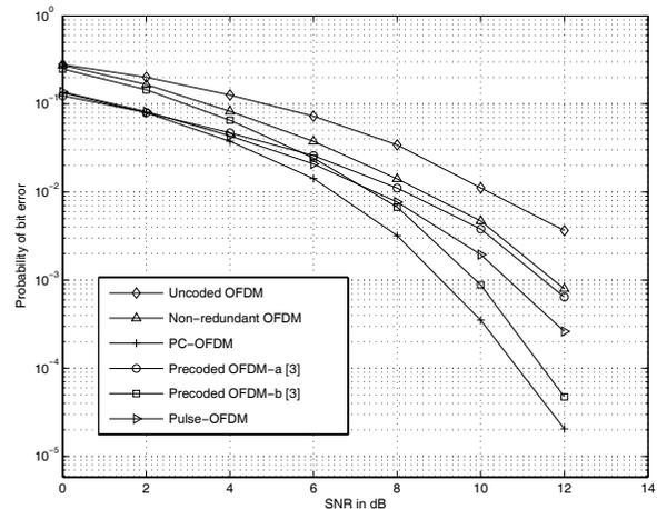
**Fig. 4.** BER of OFDM system with redundant and non-redundant coding
