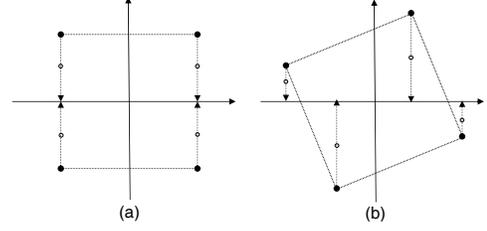
**Fig. 2.** Effect of signal space diversity on 4-PSK. (a) Without signal space diversity,  $\delta_{\min}(\underline{\mathcal{A}}) = 1$ . (b) With signal space diversity,  $\delta_{\min}(\underline{\mathcal{A}}) = 2$
