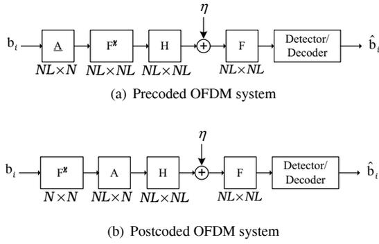
**Fig. 1.** Precoded vs. Postcoded OFDM systems
