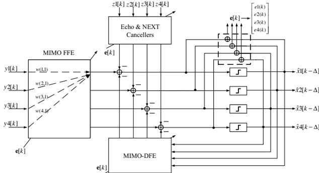
Fig. 4. Joint Cancellers and MIMO-DFE adapted structure
