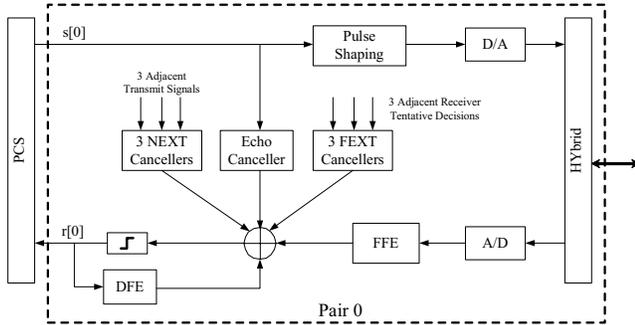
Fig. 2. Traditional 10GBASE-T transceiver block diagram
