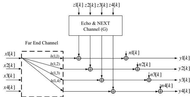
Fig. 3. Block diagram of MIMO Channel
