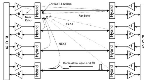
Fig. 1. 10 Gigabit Ethernet over UTP
