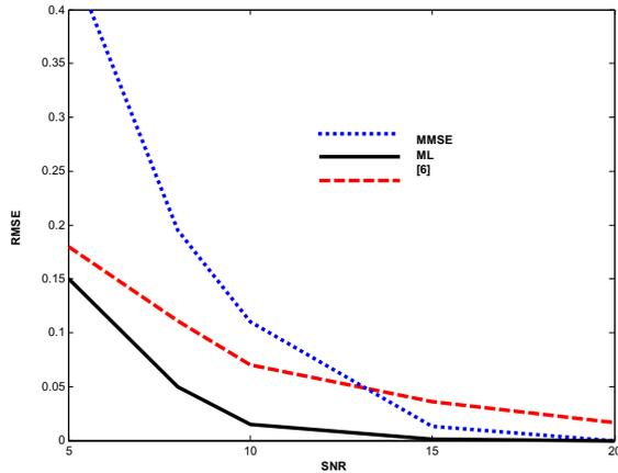
Fig.2 : Root-mean-square error (RMSE) of delay estimation versus signal-to-noise ratio
