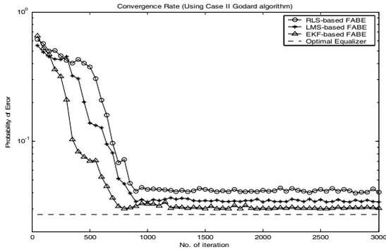
Fig.2b : Convergence rate for 3 types of FABEs using Case II Godard algorithms in a single static channel.
