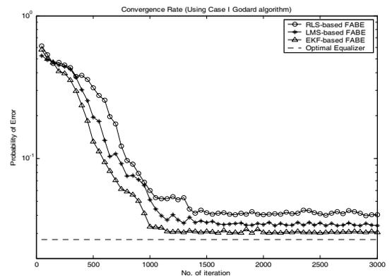
Fig.2a : Convergence rate for 3 types of FABEs using Case I Godard algorithms in a single static channel.
