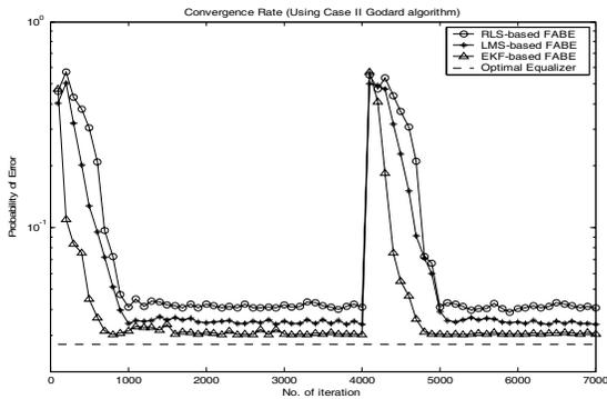
Fig.3b : Convergence rate for 3 types of FABEs using Case II Godard algorithms in changeable channels.
