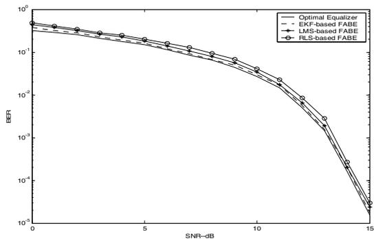
Fig. 4: The bit error rate vs. signal to noise ratio plot for the EKF-based FABE and the optimal equalizer in a single static channel.
