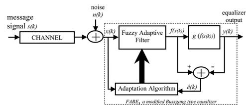
Fig 1: Powerline data transmission with fuzzy adaptive blind equalization
