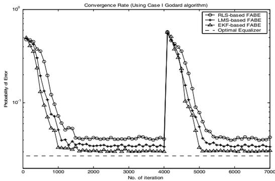
Fig.3a : Convergence rate for 3 types of FABEs using Case I Godard algorithms in changeable channels.
