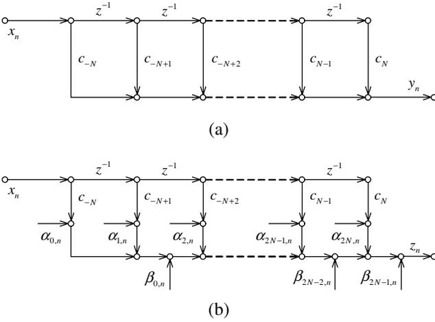
**Fig. 2.** Flow graph of a direct form I FIR filter : (a) ideal model (b) soft error model.
