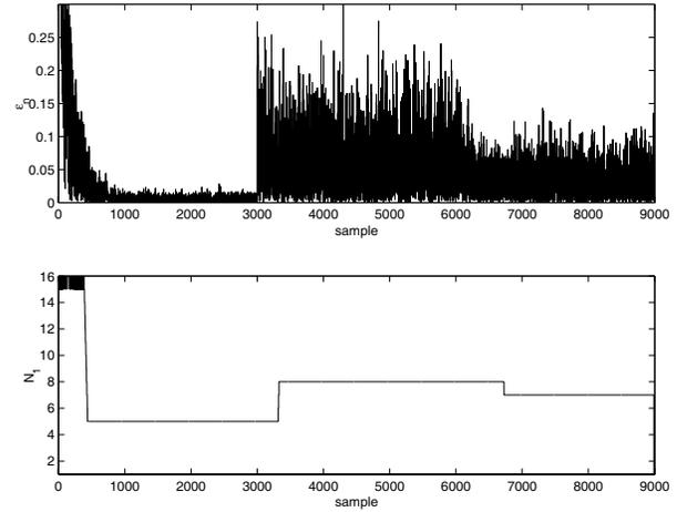
**Fig. 4.** (a) Instantaneous absolute value of error signal  $\varepsilon_n$  of the 16-tap equalizer, and (b) change of the number of coefficients  $\bar{a}$ , or  $N_1$ . The underlying channel abruptly changes at sample  $n = 3000$  and sample  $n = 6000$ .
