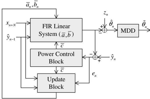
**Fig. 3.** Block diagram of soft error estimator.
