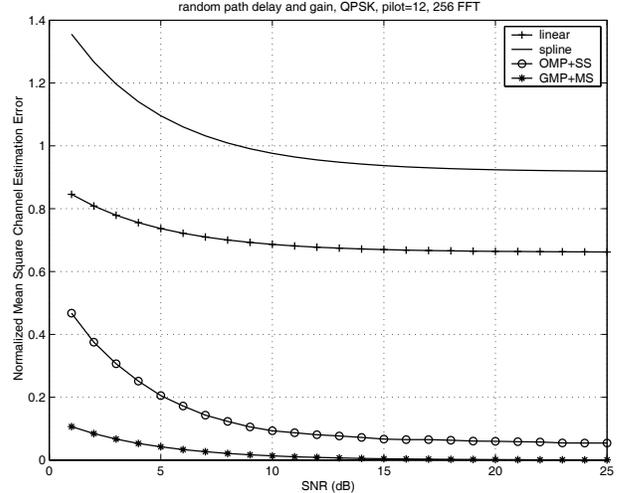
Fig. 1. Normalized mean-square channel estimation errors of different channel estimation methods, i.e.,  $(\hat{\underline{g}} - \underline{g})^H (\hat{\underline{g}} - \underline{g}) / \underline{g}^H \underline{g}$ .
