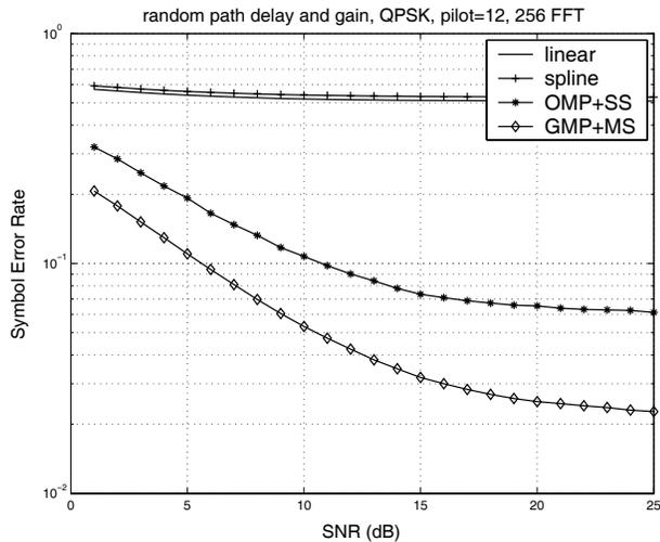
**Fig. 2.** Average symbol error rates (SERs) at data subcarriers with different channel estimation methods.
