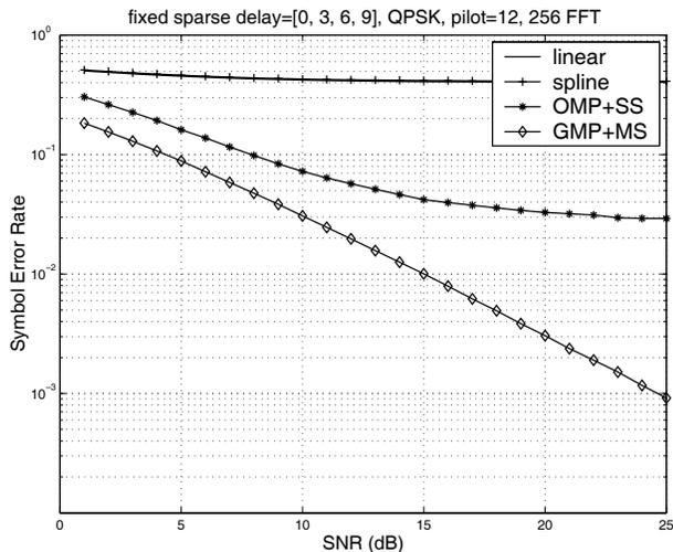
**Fig. 3.** Average SERs at data subcarriers with different channel estimation methods when multipath delay are spaced apart.
