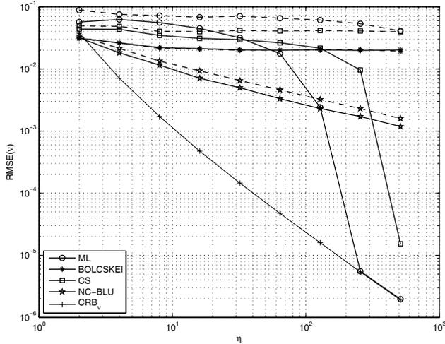
**Fig. 1.** RMSE of CFO estimators in AWGN (solid lines) and in multipath channel (dashed lines) as a function of the number of observed symbols  $\eta$ , for  $N = 4$  and  $SNR = 20$  dB.
