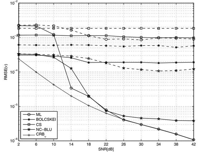
**Fig. 2.** Performance of CFO estimators in AWGN (solid lines) and in multipath channel (dashed lines) as a function of SNR for  $N = 128$  subcarriers and for  $\eta = 16$ .
