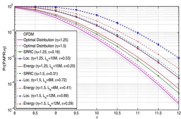
**Fig. 2.** Impact of different prototype filters and oversampling ratios on  $\epsilon_N$  and on the CCDF curves.
