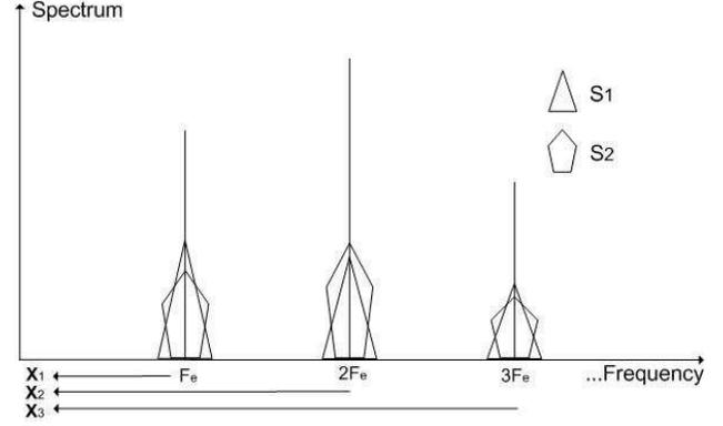
**Fig. 3.** Illustration of the gear power spectrum as well as the amplitude and frequency modulation.
