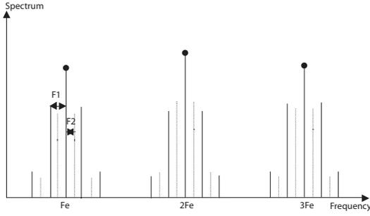
**Fig. 2.** Approximate description of the gears spectrum
