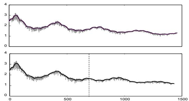
Figure 4. Experimental signals recorded for a track circuit without defect and with a defect (removed trimming capacitor)
