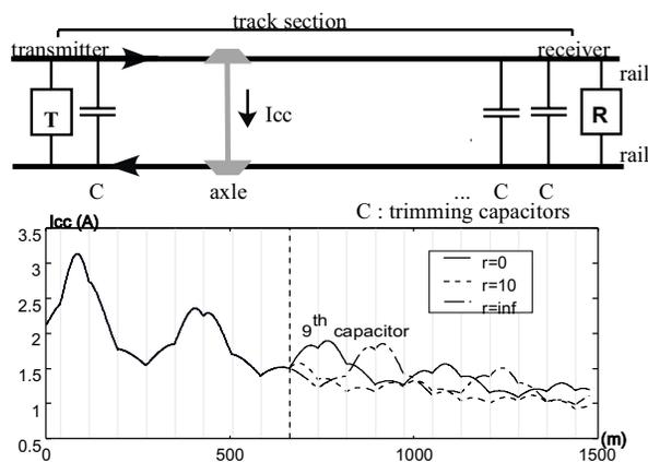
Figure 1. Track circuit representation and example of simulated  $I_{cc}$  without defect ( $r=0\Omega$ ) and with the 9<sup>th</sup> capacitor defective ( $r=2\Omega$  and  $r=\infty$ ).
