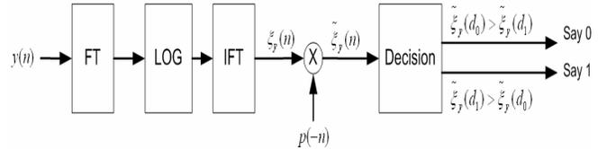
Fig. 2. Decoding procedure.
