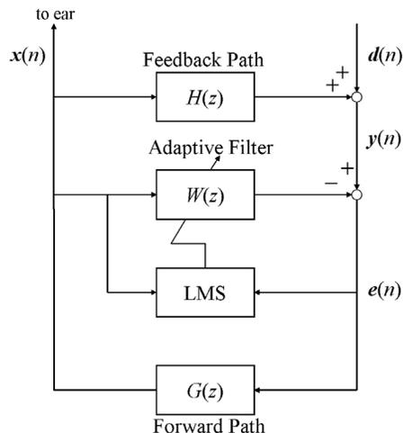
Fig. 1. Block diagram of the conventional hearing aids.
