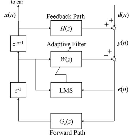
Fig. 2. Block diagram of a modified scheme by splitting the delay.
