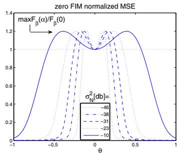
Fig. 5. zero FIM normalized MSE for Example 1. The point with the worst MSE gets closer to the zero FIM point as  $N$  increases.
