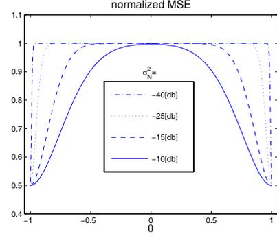
**Fig. 1.**  $h(\theta) = \theta, A = -1, a = -1, B = b = 1, g_{\theta}^{(1)}(0) = 1$ . Normalized MSE  $\left( \frac{MSE \{ \hat{\theta}_{ML} \}}{g_{\theta}^{(1)}(0)^2 \sigma_N^2} \right)$  as function of  $\theta$  for different values of  $N$ .
