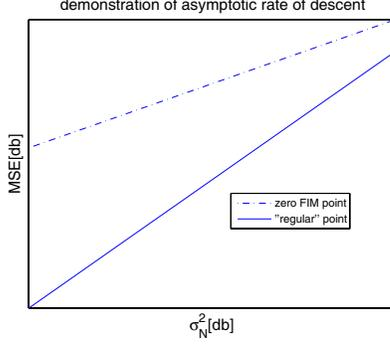
**Fig. 2.** Asymptotic MSE behavior as function of  $\sigma_N^2$  for "regular" and zero FIM points. "Regular" points exhibit a slope of 1, whereas the zero FIM point exhibits a slope of  $1 - \beta$  (the "DC level" is irrelevant here).
