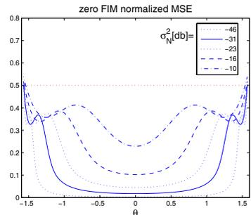
Fig. 8. zero FIM normalized MSE for Example 2. The high MSE region gets narrower as  $N$  increases.
