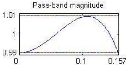
Figure 1. Magnified portion of the magnitude response in the pass-band
