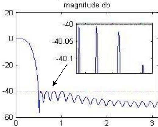
Figure 2. Magnitude response and its corresponding magnified portion in the stop-band.
