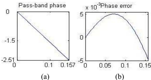
Figure 3: (a) Magnified portion of the phase response in the pass-band. (b) Phase error in pass-band.
