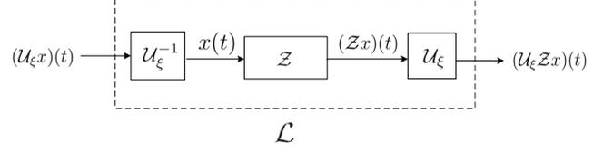
**Fig. 1.** The warping relation between the dispersive system  $\mathcal{Z}$  and the unitary equivalent narrowband system  $\mathcal{L} = \mathcal{U}_{\xi} \mathcal{Z} \mathcal{U}_{\xi}^{-1}$ .
