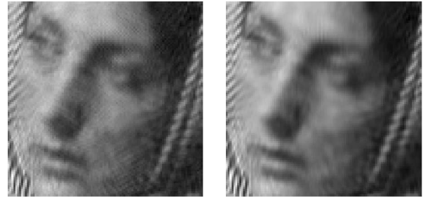
Fig. 2. Cropped versions of Barbara denoised using 4-bands wavelets: Neighblock estimator (left), proposed one using PN2 neighborhood (right).
