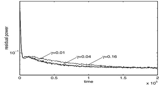
**Fig. 4.** Evolution of residual error for AP order  $L = 3$  and  $\mu = 0.125$ .
