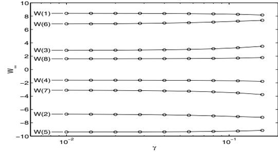
**Fig. 3.** Coefficients of  $\mathbf{w}_\infty$  versus  $\gamma$  for AP order  $L = 3$  and  $\mu = 0.125$ .
