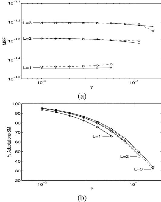
**Fig. 2.** Estimated values (—) and simulation values (---) of (a) steady-state MSE and (b) percent of adaptations versus  $\gamma$  for AP orders  $L = 1, 2$ , and 3.
