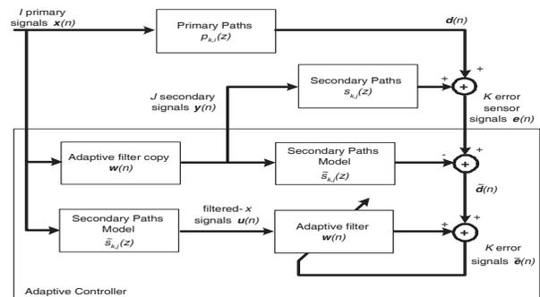
**Fig. 1.** Delay-compensated filtered- $x$  structure for active noise control.
