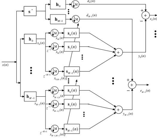
**Fig. 1.** System identification model for the subband adaptive filter for the  $M$ -subband case [4]
