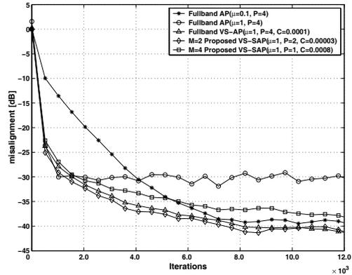
Fig. 3. Misalignment of the VS-SAP with the reduced projection order
