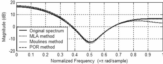
Fig. 4 Estimate of  $H_1(z)$  for SNR 20dB
