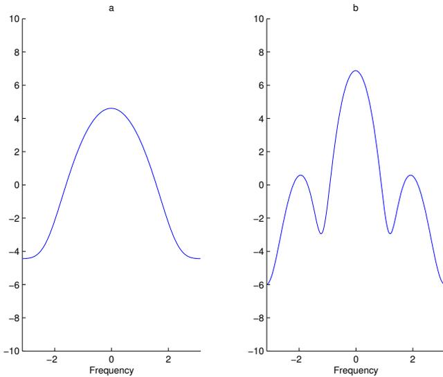
**Fig. 1.** The true log-spectra (in dB) of the two signals: (a) broadband MA signal with small dynamic range, and (b) broadband MA signal with medium dynamic range.
