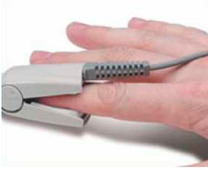
Fig. 1. DVP recorded by measuring the transmission of IR light through the finger pulp.
