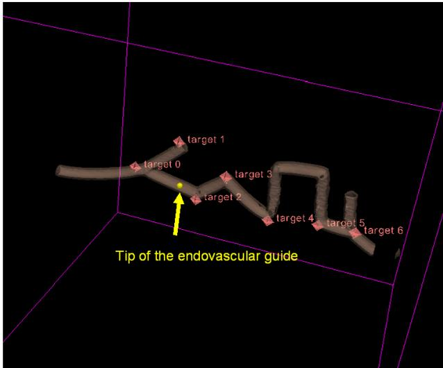
**Figure 3. Endovascular navigation to pre-defined targets. The system displays the position of the tip of the guidewire within the 3D model of the phantom vasculature.**
