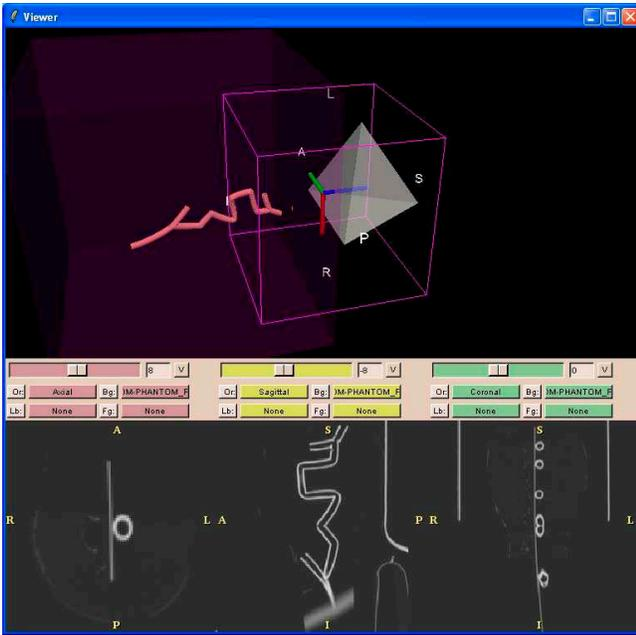
**Figure 1. Graphical User Interface of the computer assisted navigation system. The lower part of the interface displays the anatomical slices of the phantom CT dataset. The upper part of the interface shows the 3D model of the phantom vasculature registered within the reference system of the Aurora magnetic tracker, modeled as a pyramid in the scene.**
