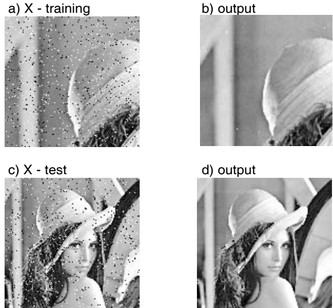
Fig. 5. Training and testing images. Results of MMNN (AGA-MOD) for Matheron decomposition by 22 dilations. (a) input for the training, (b) output by the end of the training, (c) testing input and (d) testing output.
