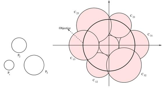
**Fig. 3.** A system of three pupils (left) and its ACS (right), the objective is represented by a thick circle.
