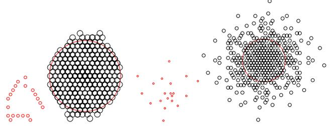
**Fig. 6.** A set of 20 pupils of unit radius with its corresponding ACS and an objective disk of radius 25. The objective is completely covered in our algorithm (left) while there are some small holes inside the objective in Golay's algorithm (right).
