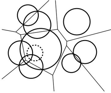
**Fig. 2.** A power diagram of 9 disks in the Euclidean plane. The dotted circle has no power cell.
