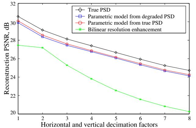
Fig. 6. Reconstruction of Lena image with Gaussian blur of  $\sigma = 1.5$ , AWGN  $\sigma^2 = 50$ , and varying decimation.
