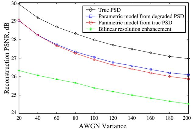
Fig. 5. Reconstruction of boat image with Gaussian blur of  $\sigma = 0.6$ , AWGN of varying  $\sigma^2$ , and (2, 2)-fold decimation.
