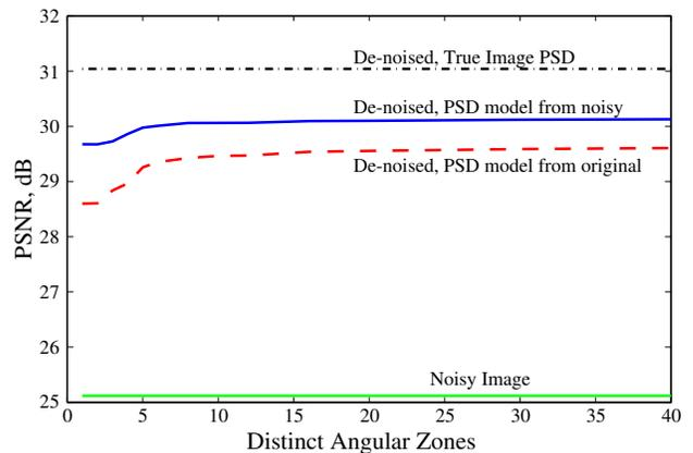
Fig. 2. PSNR of denoised boat image for varying number of angular zones. Original image corrupted by AWGN with  $\sigma^2 = 200$ .
