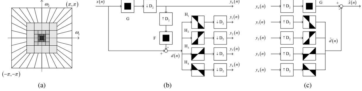
**Fig. 1.** The PDFB employed in image coding. (a) The partitioning of the frequency plane by a hybrid PDFB and wavelet decomposition, and (b) The analysis side of a PDFB; the DFB has four directional subbands and (c) the synthesis PDFB corresponds to analysis PDFB in (a).
