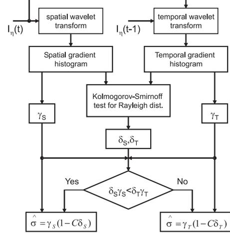
**Fig. 2.** General block scheme of the proposed noise estimation approach ( $I_\eta(t)$  and  $I_\eta(t - 1)$  stand for the current and previous input noisy frame, respectively).
