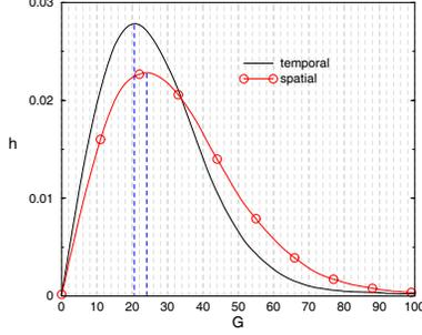
**Fig. 1.** Noise Estimation: Normalized spatial and temporal gradient magnitude histogram for the 3rd frame of “Tennis” image sequence with Gaussian noise ( $\sigma_\eta = 20$ ).
