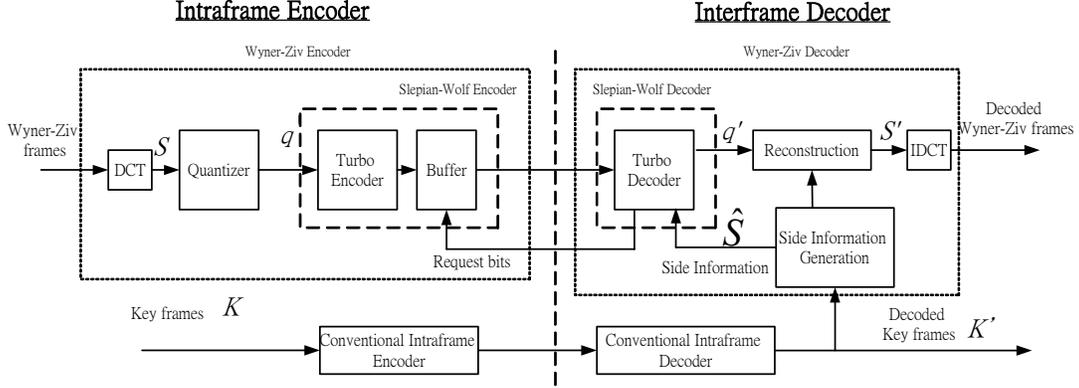
FIGURE 1. Block diagram of the proposed distributed video coding system.
