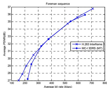
Figure 4. Rate-distortion comparison for the Foreman sequence of interframe H.263 (I-B-I-B) with the proposed DVC scheme (Key & Wyner-Ziv frames) using the coarsest quantizer ( $\bar{M}^7$ ) for the Wyner-Ziv frames and different bit-rates for the key frames.
