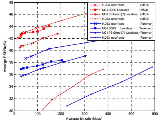
Figure 2. Rate-distortion comparison of the proposed DVC scheme with the scheme of [4,7] and H.263 for the Wyner-Ziv frames of the Foreman (solid curves) and Mother-Daughter (dashed curves) sequences with losslessly decompressed key frames for the side information.
