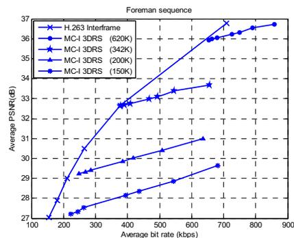
Figure 3. Rate-distortion comparison of the proposed DVC scheme (Key & Wyner-Ziv frames) and interframe H.263 (I-B-I-B) for the Foreman sequence.
