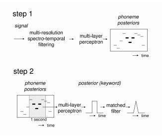
Fig. 4. Schematic diagram of the proposed technique.
