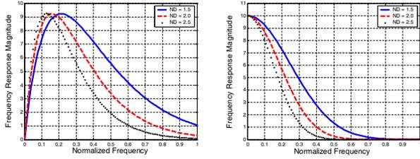
**Fig. 1.** Impulse response of longitudinal (left) and perpendicular (right) magnetic recording normalized frequency domain (normalized to sampling frequency).
