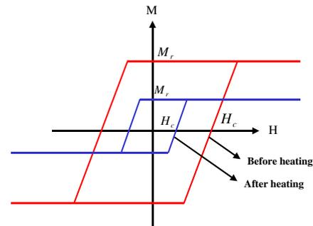
**Fig. 2.** Idealized magnetization versus magnetic field hysteresis loop (MH loop) of the medium before and after heating
