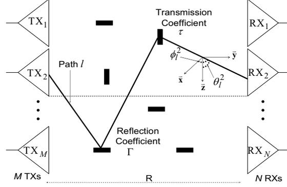
**Fig. 1.** Scattering environment with plane wave propagation. Multi-path amplitude and phase is a function of path length and the reflection and transmission coefficients of the scatterers.
