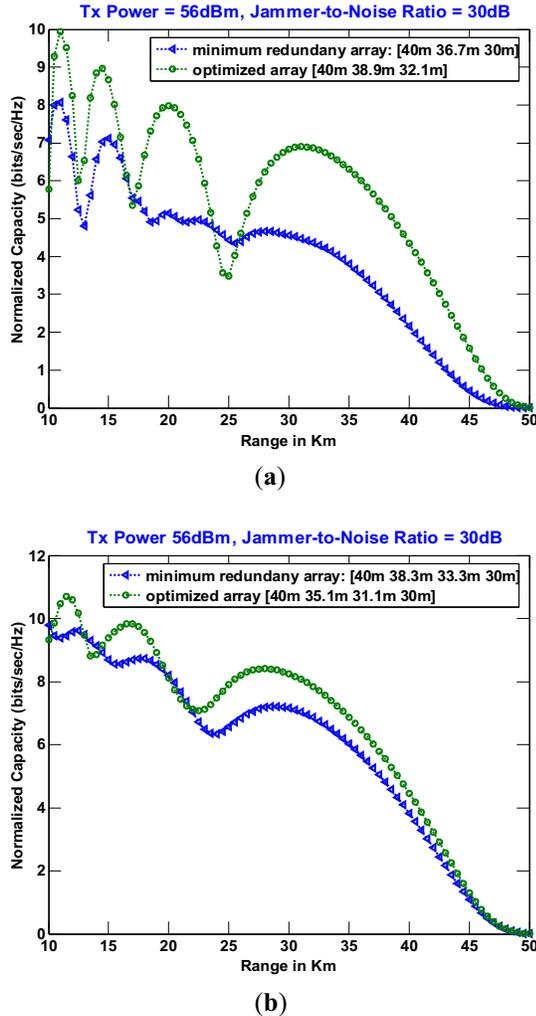
**Fig. 2.** Information-theoretic capacity of two units 10Km to 50Km apart communicating over water in the presence of one fixed and one mobile main beam jammer. (a) Three receive antennas. (b) Four receive antennas.
