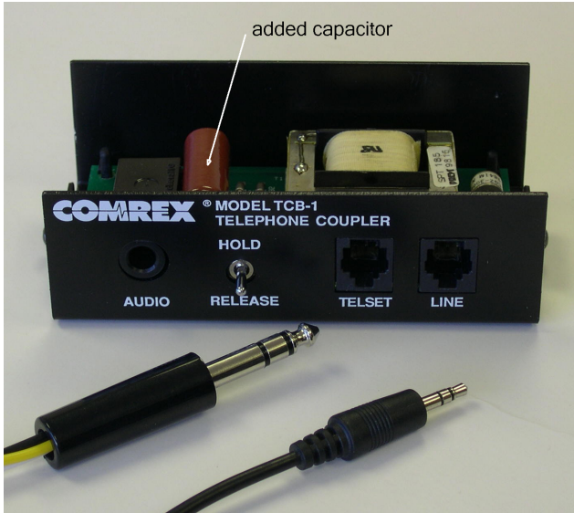
Fig. 1. Photograph of the modified Comrex model TCB-1 telephone coupler (cover removed). The audio cable (1/4-inch plug to 1/8-inch plug) shown in the foreground is used to connect the telephone coupler to a PC's sound card.
