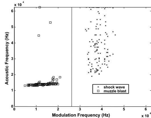
**Figure 6. Spectral extent features from the shock waves (crosses) and muzzle blasts (squares). A simple linear threshold may be used to distinguish the transient classes in the feature space.**
