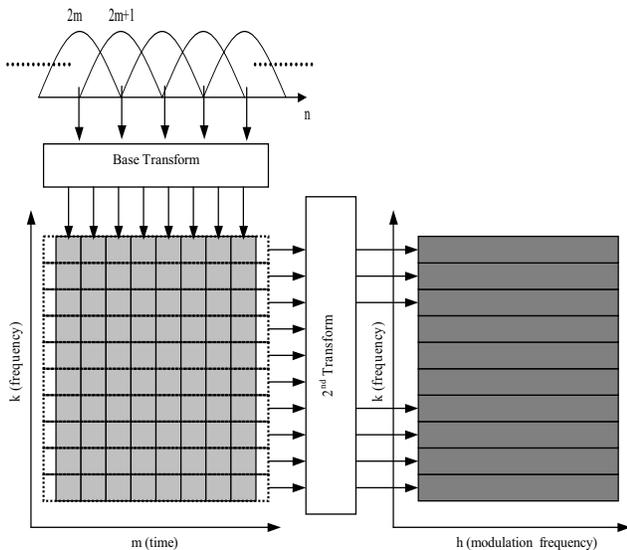
**Figure 2. Simplified structure of the two-dimensional transform.**
