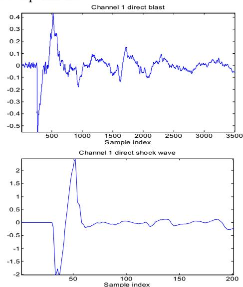
Figure 1. Acoustic transients from sniper fire: muzzle blast (above) and shockwave (below).
