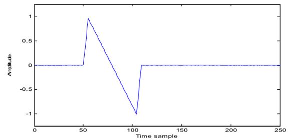
**Figure 3. A synthesized shockwave, modeled as an N-wave, with  $t_{on}=5$  samples,  $t_0=50$  samples, and  $t_{off}=5$  samples**
