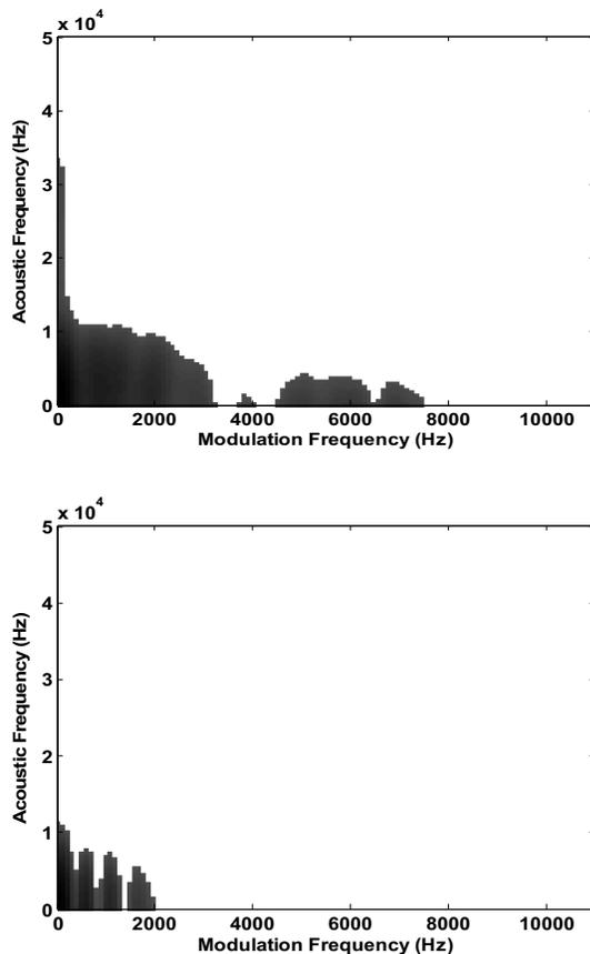
**Figure 5. Preprocessed MS corresponding to those shown in Figure 4. The MS for the shock wave (top) clearly extends further in both acoustic and modulation frequency than that for the muzzle blast (bottom).**
