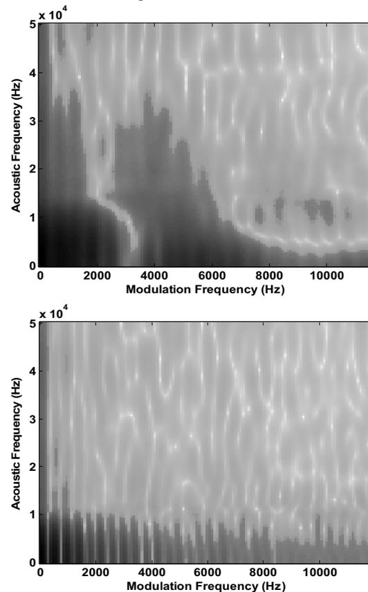
Figure 4. Modulation spectrum representations of shockwave (top) and muzzle blast (bottom).
