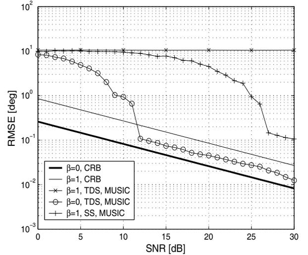
Figure 2: Performance of the TDS-MUSIC algorithm with orthogonal ( $\beta = 0$ ) and coherent ( $\beta = 1$ ) signals, compared to the spatial smoothing-MUSIC and CRB.
