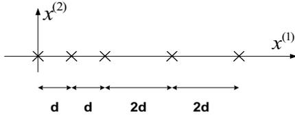
Figure 4: Non-uniform linear array;  $d = \lambda/2$
