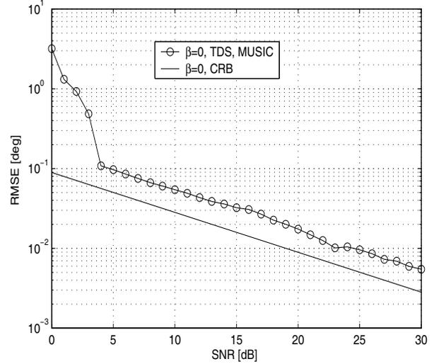
Figure 5: Performance of the TDS-MUSIC algorithm with orthogonal ( $\beta = 0$ ) signals using non-uniform array, compared to the CRB.
