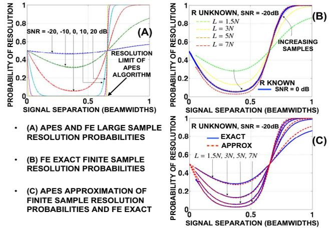
Fig. 2. APES and FE Probability of Resolution for  $N = 24$  element ULA
