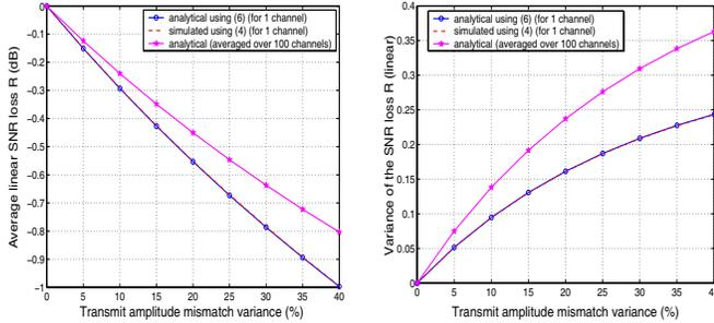
Fig. 2. The average (in dB) and the variance (in linear units) of the SNR loss  $R$  in the presence of transmit amplitude mismatches
