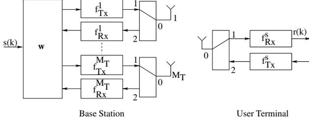
**Fig. 1.** The transmit-MRC MISO system including the RF transceiver responses
