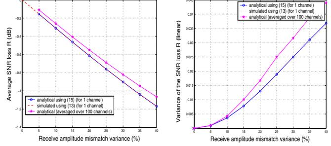
Fig. 4. The average (in dB) and the variance (in linear units) of the SNR loss  $R$  in the presence of receive amplitude mismatches
