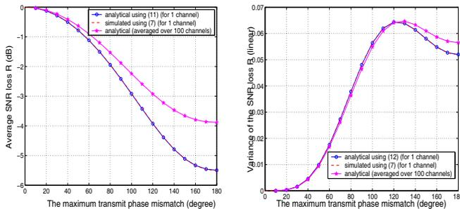
Fig. 3. The average (in dB) and the variance (in linear units) of the SNR loss  $R$  in the presence of transmit/receive phase mismatches
