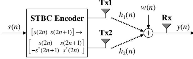
Fig. 1. Space-time block coded transmission diagram.
