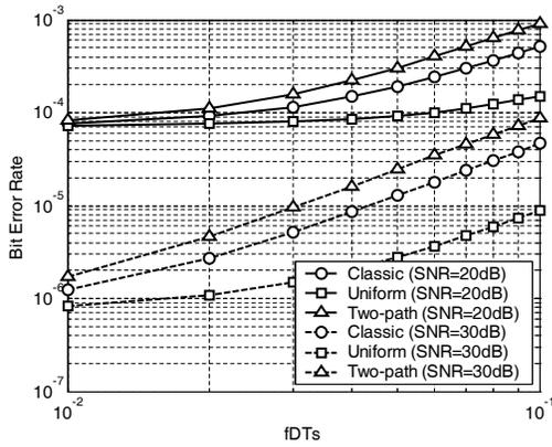
Fig. 3. Comparison of analytical and simulated BER of decision feedback detector with different level of correlation.
