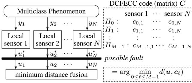
Fig. 1. Distributed classification system architecture
